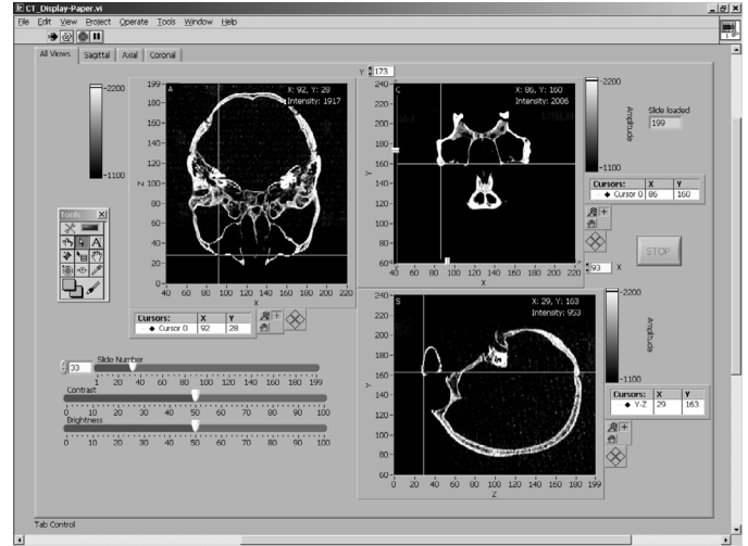
Fig. 11. Software front panel showing the axial, sagittal, and coronal views of the human skull used in the fluid detection experiment.
